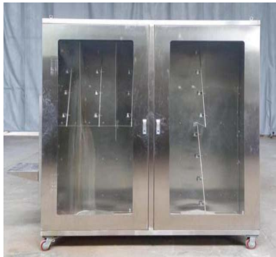
Figure 2.1 Hidden Fire Test Chamber
