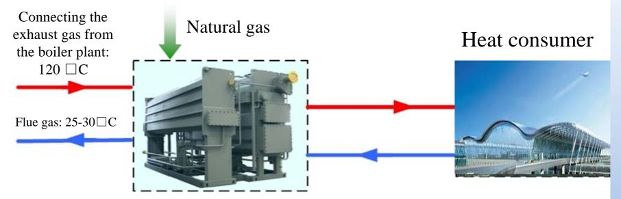
Residual heat reclaiming unit for gas boiler plant
