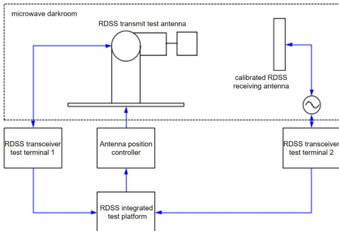
Figure 2 Construction of the transmit EIRP test environment
