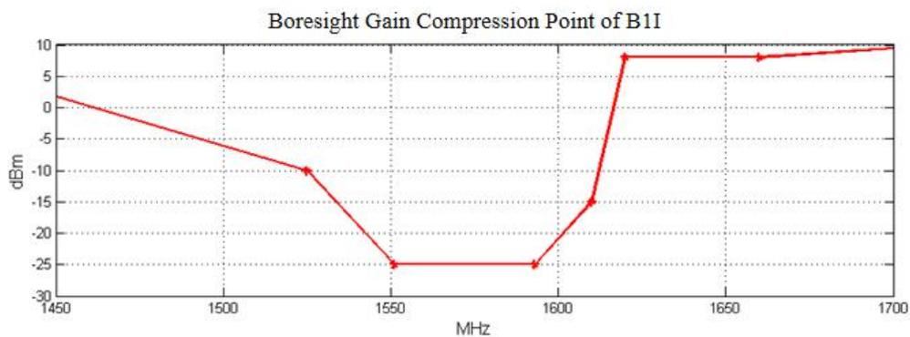
Figure 2-2 Minimum Input 1 dB Gain Compression Point vs. Frequency
