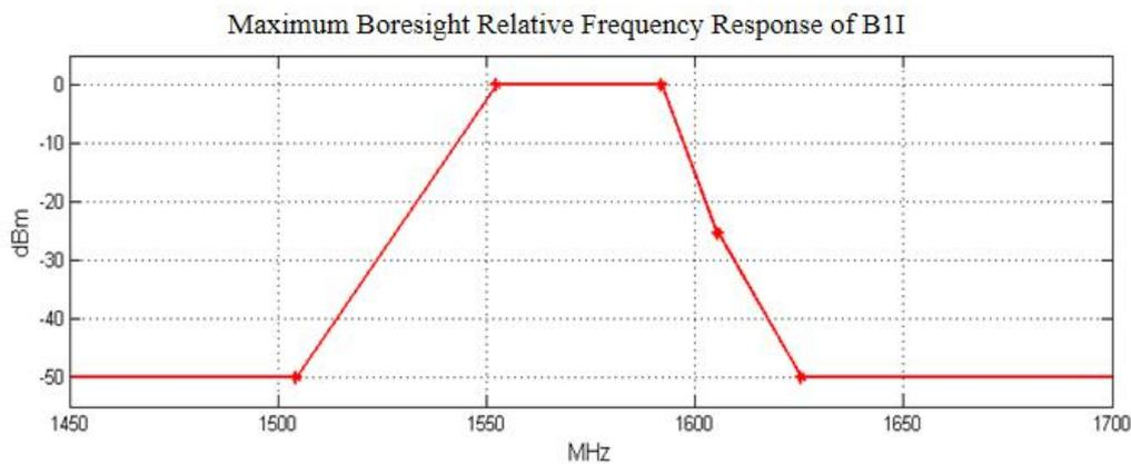
Figure 2-2 Maximum Boresight Relative Frequency Response
