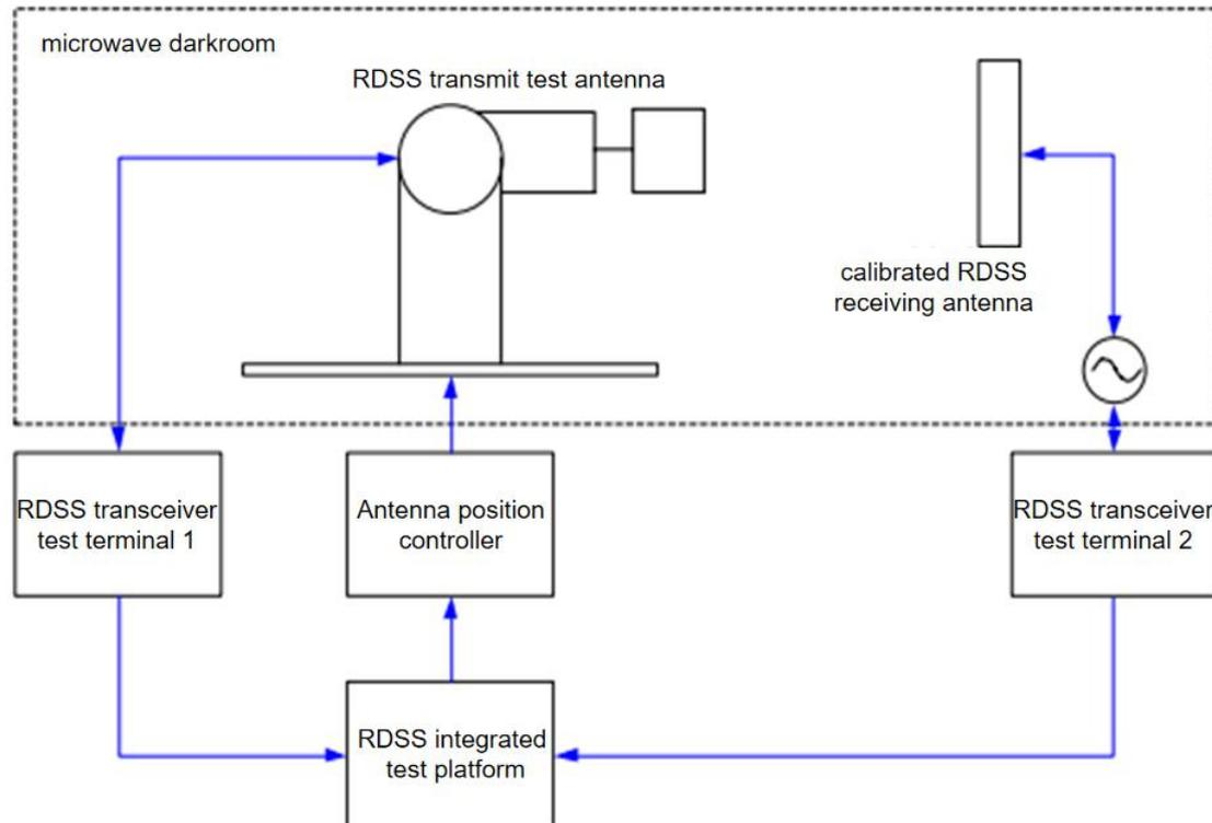
Figure 1 Construction of the transmit EIRP test environment
