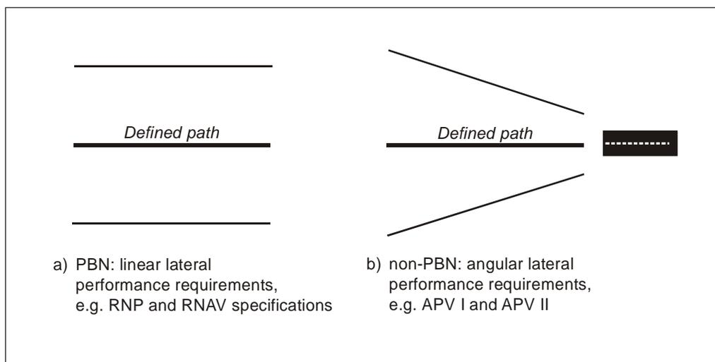
Figure I-A-1-2. Lateral performance requirements for PBN
