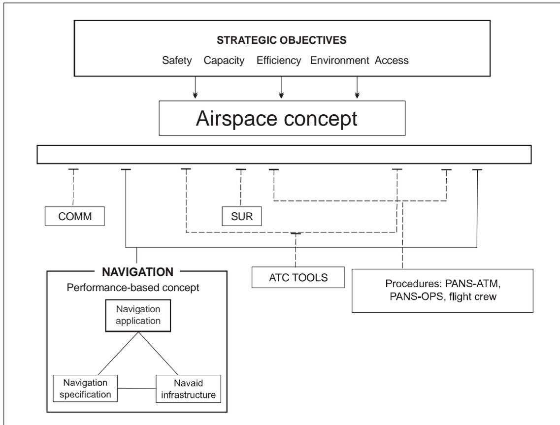
Figure I-A-2-2. Relationship: Performance-based navigation and airspace concept
