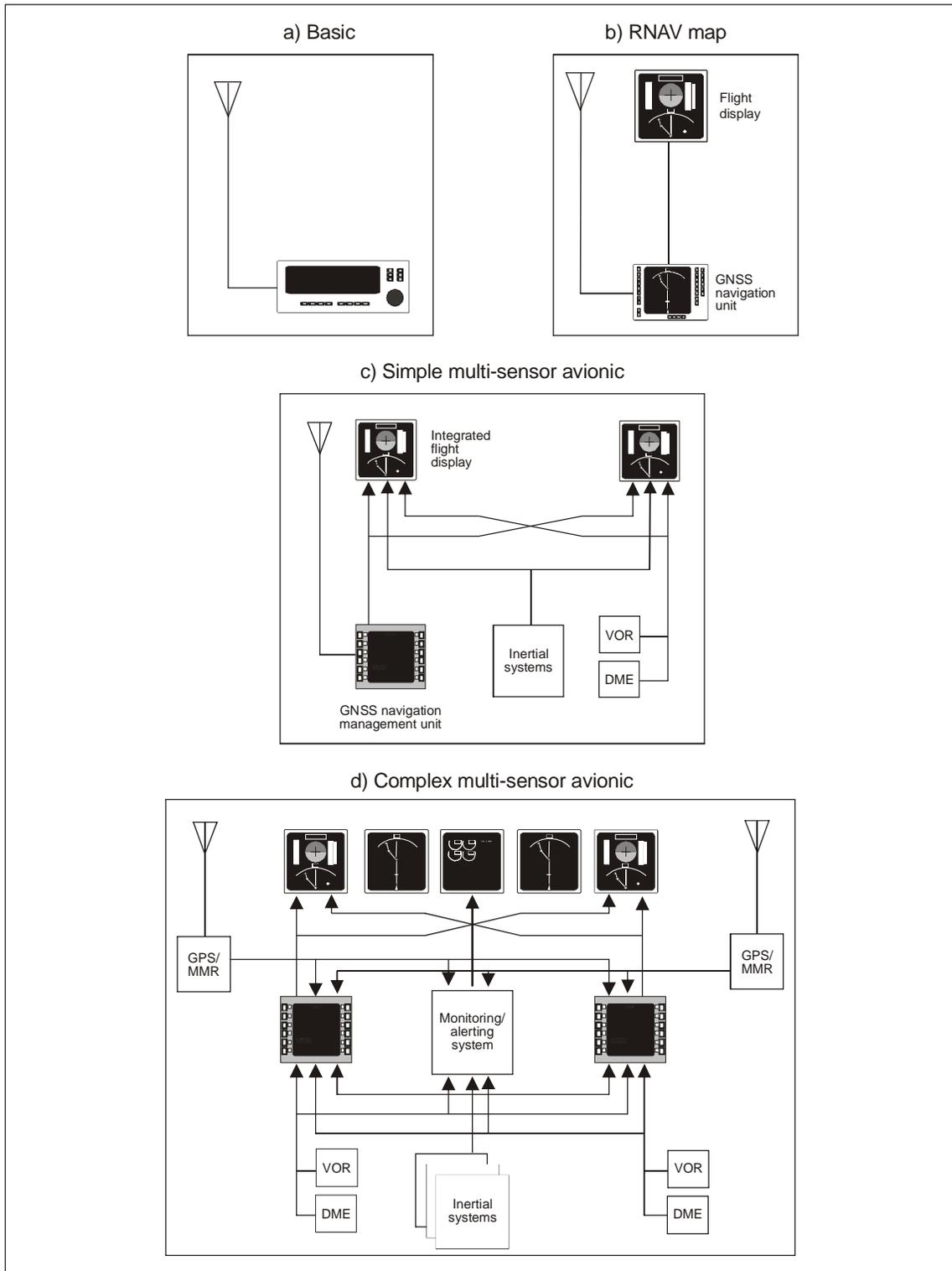
FIGURE I-A-A1-2. RNAV systems — from basic to complex
