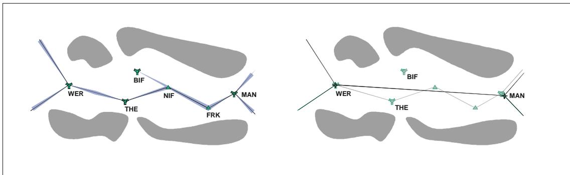
Figure I-A-A1-1. Navigation by conventional navigation compared to RNAV
